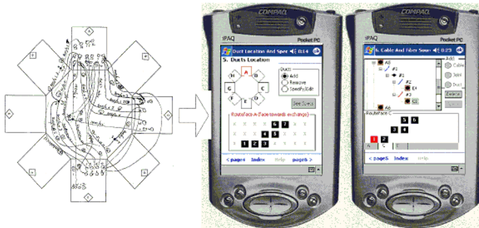
Fig 3: Manual (Left) and Electronic (Right) interface for the topographic view of a UUC cable network
