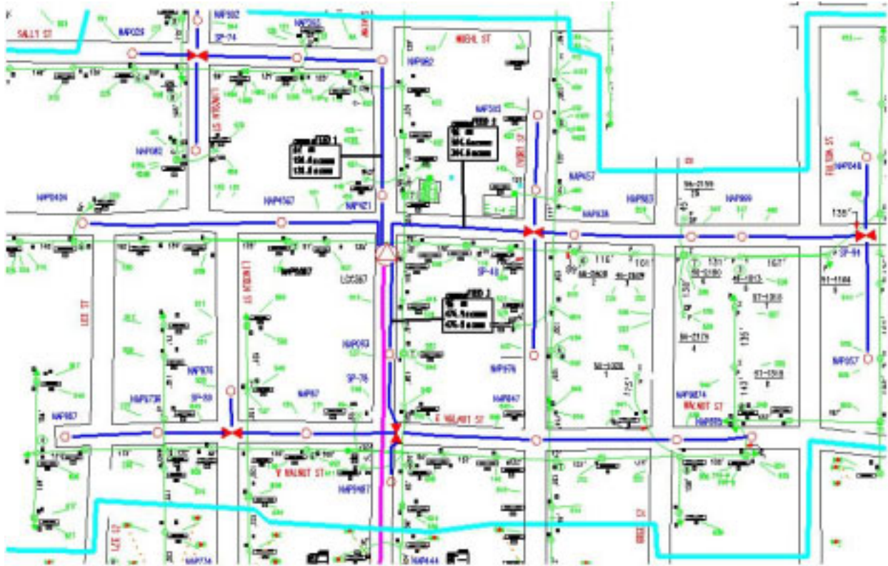
FTTH cabinet serving area showing the node, splices, pedestals and fiber cable
