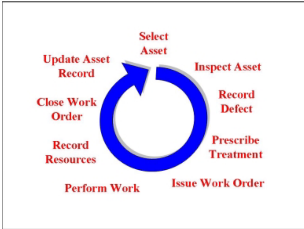
Figure 2: Asset-based Work Management Process
